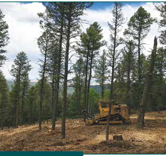
Masticator working in a fuels treatment area. Photo: CSFS
